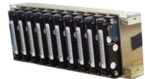
Sturdy lightweight, milled-aluminum canister records up to 10 TB and is designed for quick data transfer to ground stations from mobile vehicles. Interior view at right shows the 10 disk drives in the canister.
