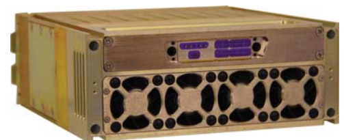
Rear view of canister shows high speed SAS 6 Gb connectors and four variable speed, high performance cooling fans.
