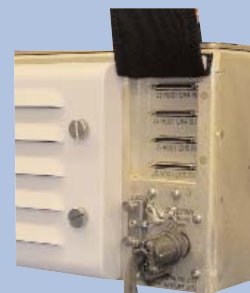
Rear view of recessed I/O panel with protective rain flap.
