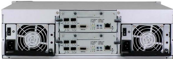
SX-3418R base unit holds 16 drives and offers eight 8 Gb F/C host connections to create a virtual "SAN-In-A-Box."
