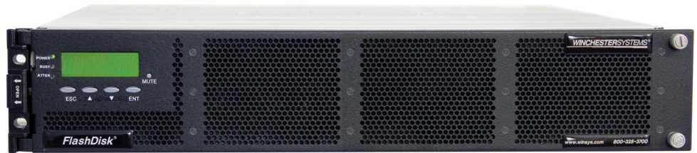
FlashDisk DBA clocks in at 73,000 sustained random and 213,000 sustained sequential IOPS with bursts to 500,000 IOPS using typical database-sized 4 KB blocks.
