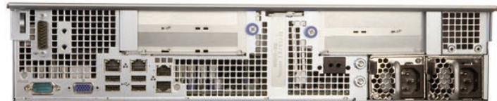
Rear view of FlashServer FS-2600 showing one external PCIe x16 (center) and four PCIe x8 slots. Configurations of up to three external PCIe x16 slots are also available.
