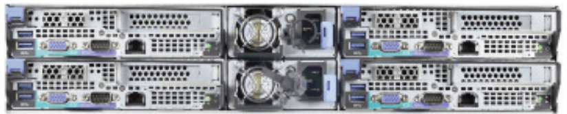
Each of the four servers are field replaceable without interrupting the other three servers running. The power supplies, fans and 24 disk drives are hot swappable.
