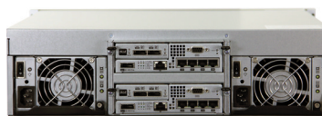
RF-3U16 with 4 SAS 6Gb ports plus 8 iSCSI 1GbE ports.
