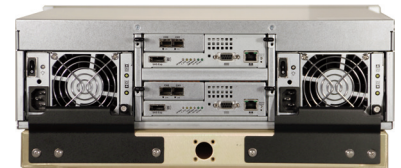
FlashDisk RF-3U16 rear view with 1U mounting tray and secure power supply clamps.
