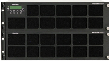
The RF-3U16 Series scales to 1,920 TB with 14 optional 3U16 expansion shelves using a total of 240 disks with 8 TB each.
