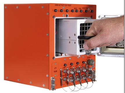
Sturdy, lightweight aluminum canister records up to 19.2 TB using 24 SSDs and is designed for quick data transfer to ground stations from mobile vehicles. The canister connects to the chassis with a military grade connector designed for 10,000 insertion cycles.
