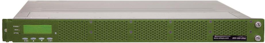
*FlashDisk RV-1300 disk arrays feature 2.5" SAS or SSD disks and are ideal for mobile applications - providing field reliability and data protection at COTS prices.*
